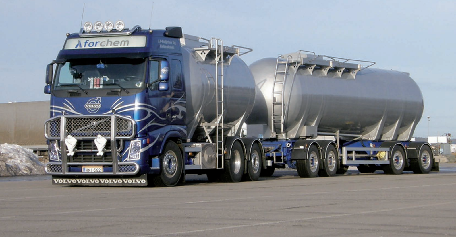
Composite sandwich truck tank by Muovityö Hiltunen OY: the reduced tank weight allows a payload increase of 10%
