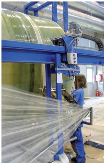
Filament winding of a sandwiched tank
